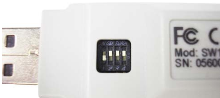
Setting for Swifty switch interface.
